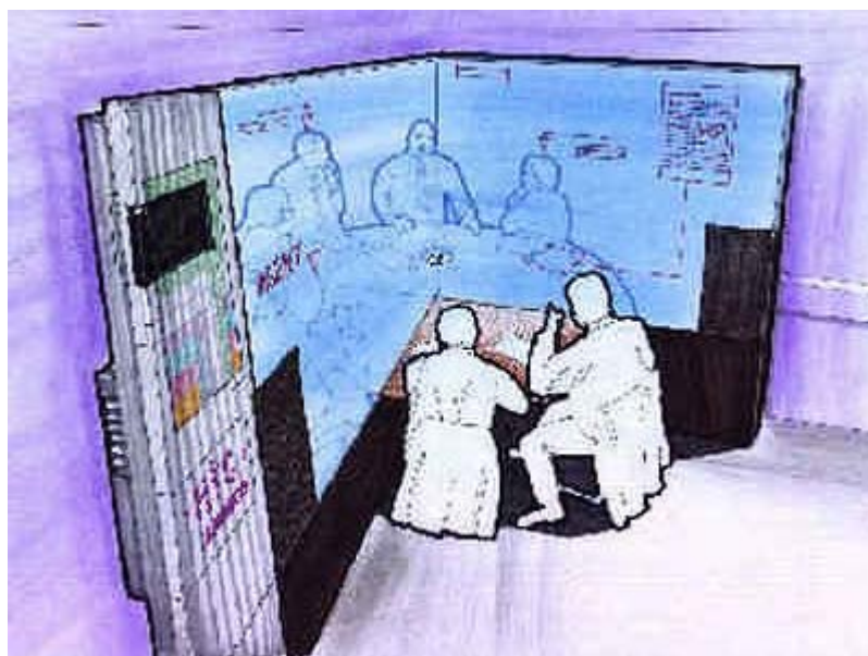
Immersive telepresence in virtual video-conference systems. Life-size communication partners meet around a desk, half virtual and half real.
